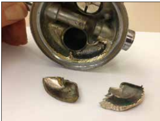
Figure 9. Two “venturi’s” removed from KM 350 regulators illustrating their flow noise generating configuration.
