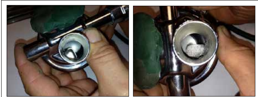
Figure 7. Airflow exit from venture without and with felt metal screen
