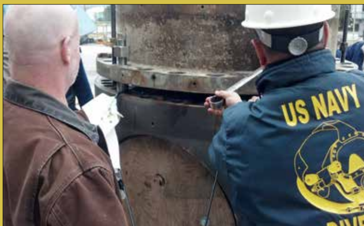
Mr. Jim Peck (left) and NDC Josh Miller working O-ring replacement procedure on Non-RFI hub.
