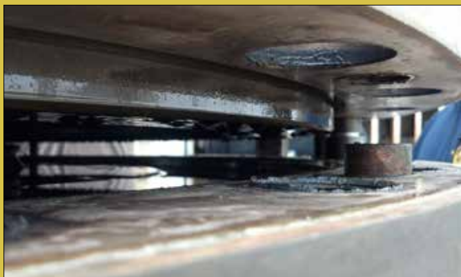
Hub cone could only be separated two inches from hub; tight but manageable for the divers; O-ring groove is visible.
