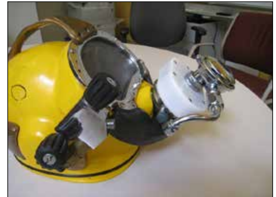
Figure 8. Proof-of-principle expansion chamber
