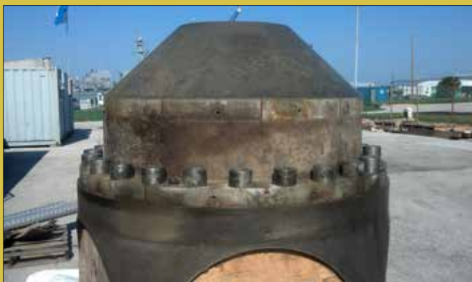
Non-RFI hub that was used to practice O-ring replacement procedure.
